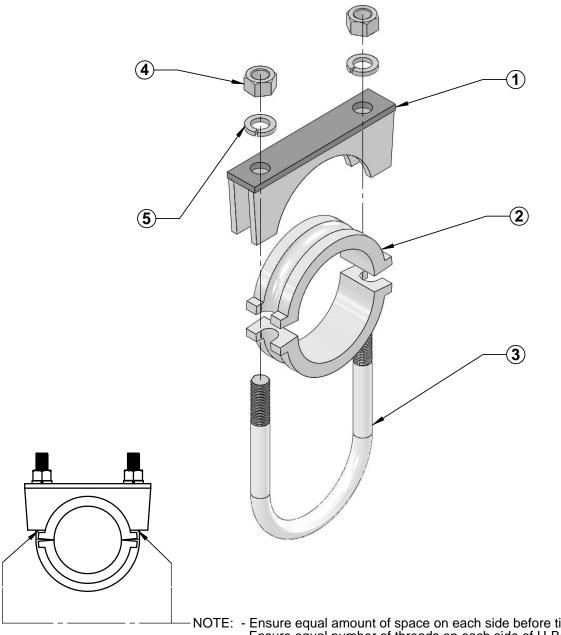
NOTE: - Ensure equal amount of space on each side before tightening U-Bolts .
